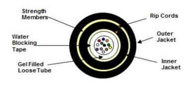
(Representation of a standard 12 fiber construction)
