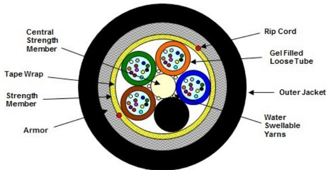
(Representation of a standard 48 fiber construction)
