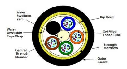
(Representation of a standard 48 fiber construction)
