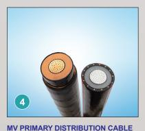
MV rated 35kV with TRXLPE insulation and XLPE jacket, with AL or CU conductors; used for runs to transformers. Features "Discharge-Free" design.
