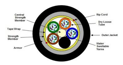
(Representation of a standard 48 fiber construction)
