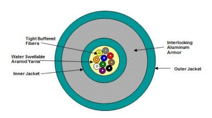
(Representation of a standard 12 fiber construction)
