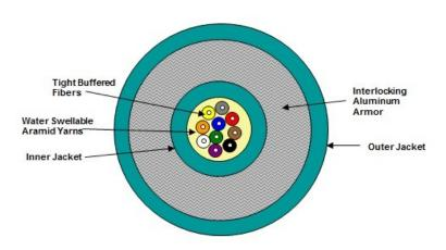
(Representation of a standard 12 fiber construction)
