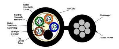
(Representation of a standard 48 fiber construction)
