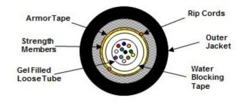
(Representation of a standard 12 fiber construction)
