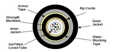
(Representation of a standard 12 fiber construction)
