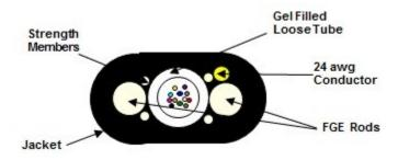
(Representation of a standard 12 fiber construction)
