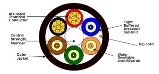
(Representation of a standard 4 fiber construction)
