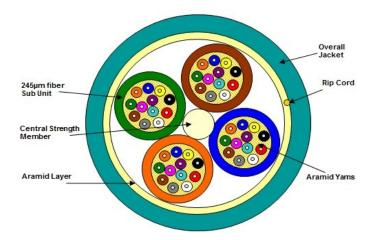
(Representation of a standard 48 fiber construction)
