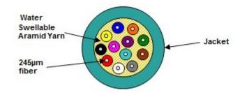
(Representation of a standard 12 fiber construction)
