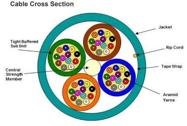
(Representation of a standard 48 fiber construction)
