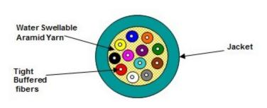
(Representation of a standard 12 fiber construction)
