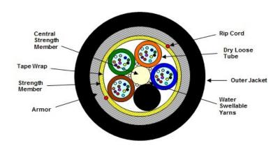
(Representation of a standard 48 fiber construction)
