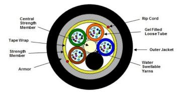
(Representation of a standard 48 fiber construction)
