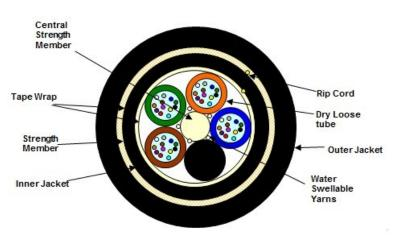
(Representation of a standard 48 fiber construction)
