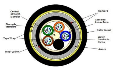
(Representation of a standard 48 fiber construction)
