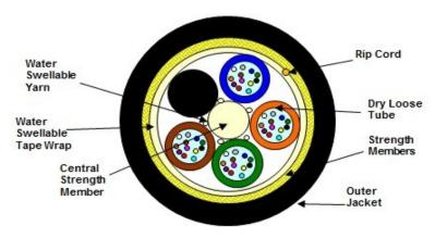
(Representation of a standard 48 fiber construction)
