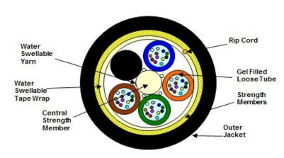
(Representation of a standard 48 fiber construction)
