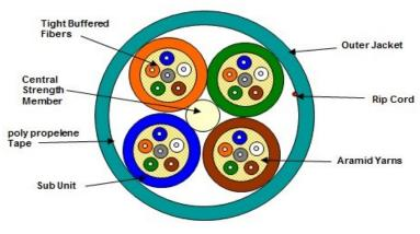
(Representation of a standard 48 fiber construction)
