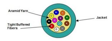
(Representation of a standard 12 fiber construction)
